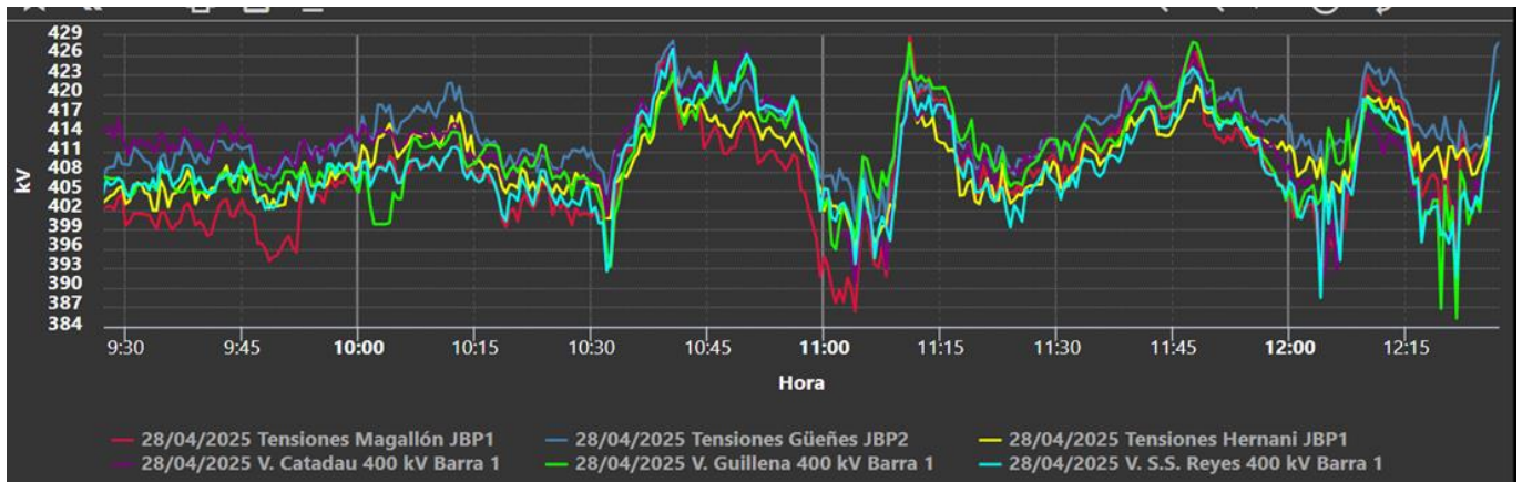
Figure 2. Voltage in 400 kV transmission network from 09:30 to 12:30 h
